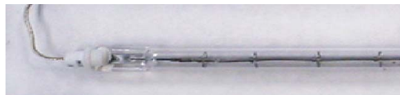
Tungsten in a quartz envelope
