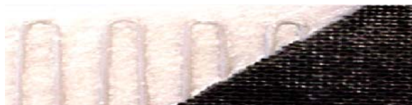
Embedded - resistance alloy
